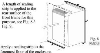
the sealing should provide a complete isolation of the appliances combustion system from the vehicle interior
