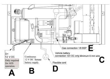
The refrigerator is equipped with two 12 volt DC connections and one D+ connection ( D+ is only required if automatic function has been preset )
