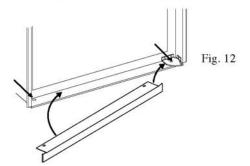
(The hinge plate can be on the right or left side depending on the door swing.)
